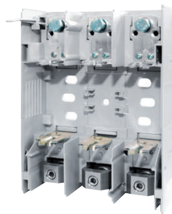
RBK 1VD-M for installation on mounting plate, picture of fuse switch disconnecter without fuse links cover and terminal shrouds, top cable terminal - M screws, bottom cable terminal - V-clamps, (RBK 1 VG-M - bottom cable terminal - M screws, top cable terminal - V-clamps)
